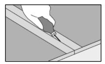
Apply the cold welding liquid by pressing the needle deeply into the seam Ensure you apply enough liquid along the entire joint.
