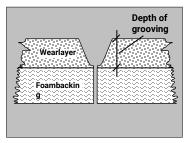
The grooving depth of seams must never be deeper than 2/3 of the thickness of the wear layer.
