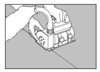
The joints are chamfered or grooved to about 2/3 of the compact thickness using a hand grooving tool or machine prior to welding. Never reach the foam backing when existing.
