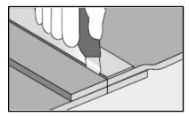
The sheets can be cold welded 24 hours after installation. Overlap the two sheets till the pattern match is achieved. The overlapping will be double cut in one step or two in case of thick flooring alongside a metal ruler. The result shall be an extremely tight joint.
